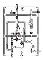
HBP High temperature by-pass flush with locking ball valve
