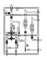
2 PUMPS H High temperature loop recirculation pump
